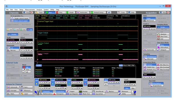
Timing diagram for external triggered mode (2 µs period of external signal)
